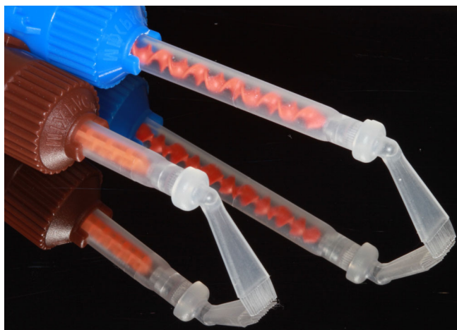
FIGURE 1 Self-mixing tips employed in this study. The Helical mixing tip (blue, Sulzer) is a conventional tip commonly used in dentistry. On the other hand, the T-Mixer mixing tip (brown, Sulzer) features an innovative design that aims to break up and rearrange fluid elements within the mixer geometry. This design allows the T-mixer mixing tip to achieve a more efficient mixing process using the same number of elements but in a considerably shorter length.
