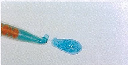
Fig. 4 After a mixing tip is attached, a small amount of gel is dispensed onto a mixing pad.
